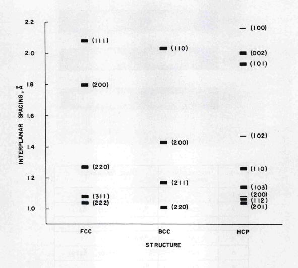
Figure 6. Schematic representation of the diffraction patterns given by three phases of iron, showing the limited number of diffraction lines where overlap does not occur.
